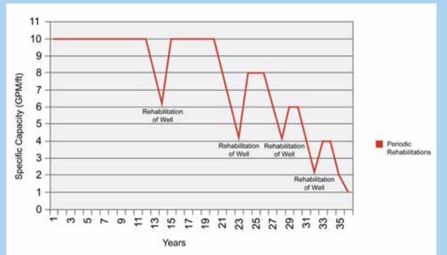
most wells will experience progressively shorter run cycles between rehabilitations, eventually leading to well failure (see figure above).
